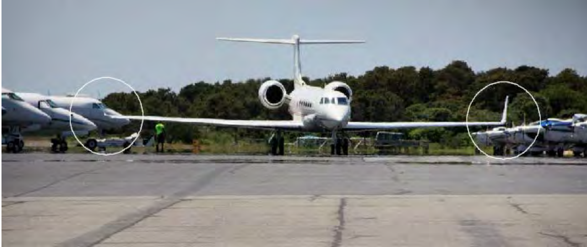
Figure 2-16 – Constricted Taxilane Width – South Ramp
